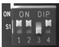
E - probe connected. Probe correction -2°C
